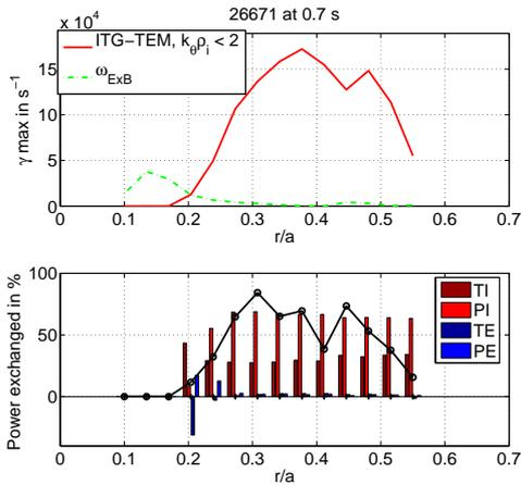
Figure 3: Growth rate of drift modes and power exchanged with plasma particles
