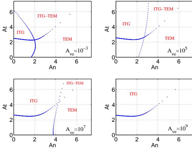
Figure 2: Stability threshold of drift electrostatic modes ( $k_{\theta}\rho_i \sim 0.4$ ) computed for different values of the collisionality parameter  $A_{ve}$ : the areas without any label are stable regions of the  $(A_n, A_t)$  plane.
