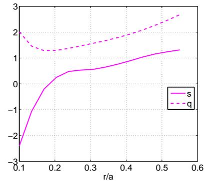
Figure 4: Safety factor  $q$  and magnetic shear  $s$  for pulse 26671.
