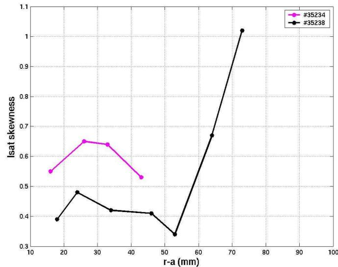
Figure 3 The radial profile of  $I_{\text{sat}}$  skewness in the SOL
