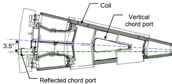
Fig. 4 – Top plan of chord port implantation
