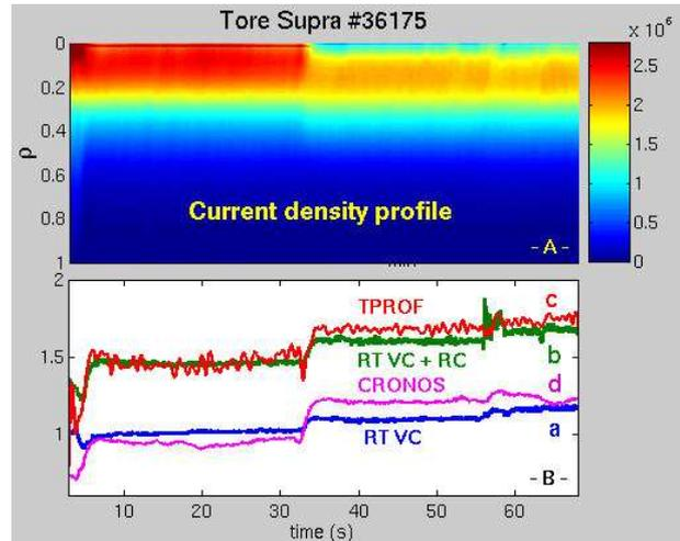
Fig. 6 – A - Current density profile given by CRONOS code and- B - Evaluation of the minimum of the safety factor  $q$  a) in real time with the traversing chords only, b) in real time with the new chords, c) by TPROF inversion with the ten chords, d) given by CRONOS code
