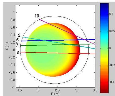
Fig. 5 –  $B_T$  poloidal component (in T) due to the toroidal ripple in the incident plan of the reflected chords
