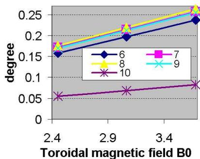
Fig. 6 – Ripple correction to polarimetric angles of reflected chords
