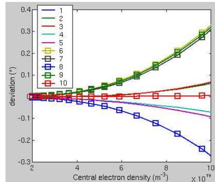
Fig. 3 - Cotton-Mouton effect in degree on the polarimetric angles vs central electron density
