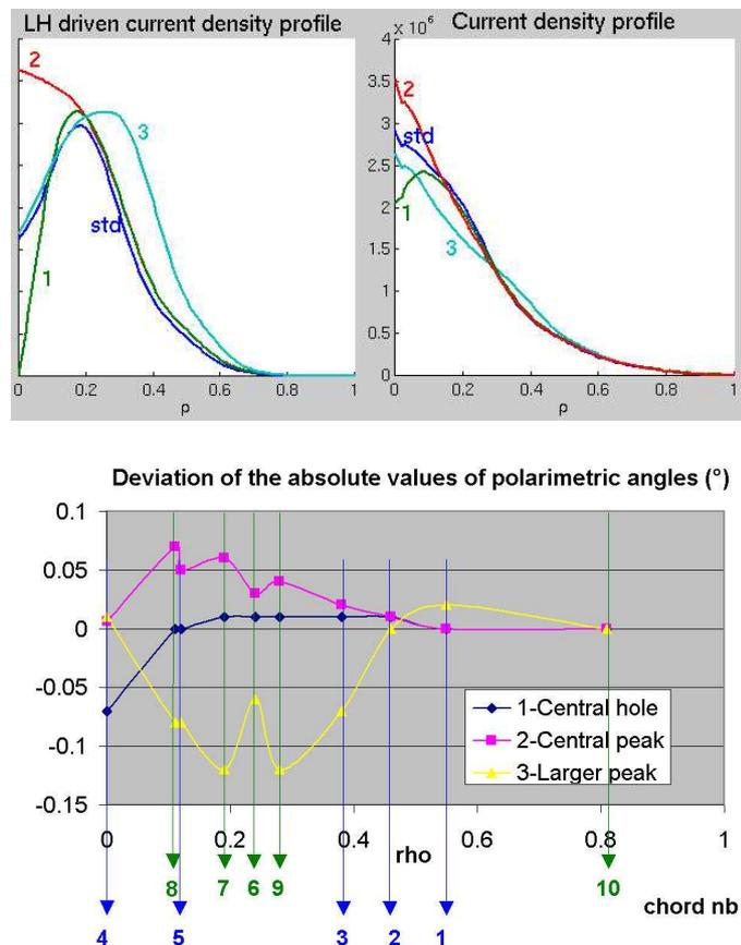
Fig. 7 – Different shapes of LH driven current density profile used in CRONOS code and deviation of the absolute values of polarimetric angles in degree for various shapes of LH driven current density profile
