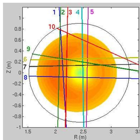
Fig. 2 – Position of the traversing and the reflected chords.
