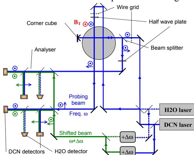
Fig. 1 – The Tore Supra interfero-polarimeter
