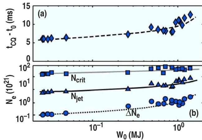
Fig. 3. (a) Time between jet trigger and start of CQ and (b)  $N_{\text{crit}}$ , minimum theoretical number of electrons for CQ collisional RE suppression,  $N_{\text{jet}}$ , actual number of delivered bound electrons at start of CQ, and  $\Delta N_e$ , observed free electron rise at start of CQ; all as a function of initial plasma thermal energy  $W_0$ .
