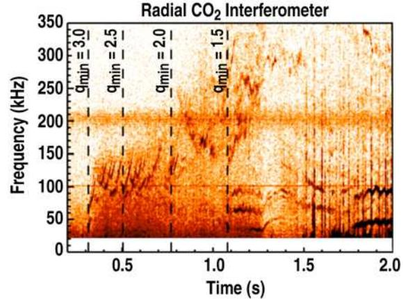
Fig 3. Spectrogram of the  $\text{CO}_2$  interferometer signal showing the Alfvén cascades and the values of  $q_{\min}$  inferred from them [7]. Lower frequency tearing modes are also observed beginning at 1.1 s.
