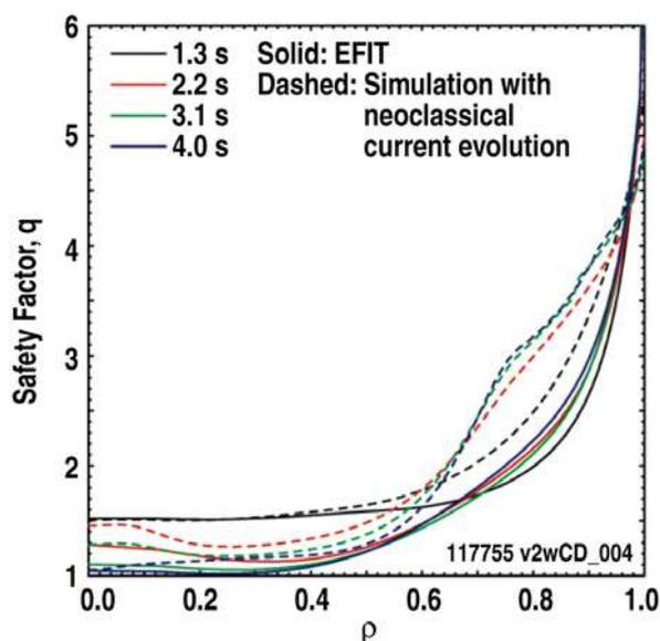
Fig. 4. Comparison of  $q$ -profiles from EFIT (solid lines) with those the CORSICA simulation with neoclassical current diffusion (dashed lines). The initial simulation and EFIT profiles differ because the former includes the kinetic pressure.
