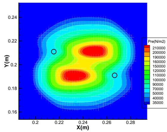
Figure 2.d Contours of pressure profile at 65.6 μs.
