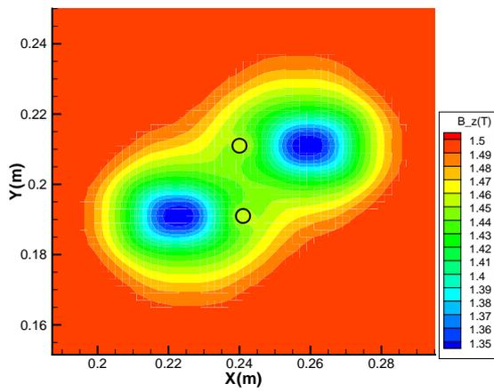
Figure 2.c Contours of magnetic field ( $B_z$ ) at 41 μs.
