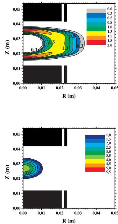
Figure 2: Density profiles of the dust ( $\times 10^{10} \text{m}^{-3}$ ) (top) and electrons ( $\times 10^{15} \text{m}^{-3}$ ) (bottom).
