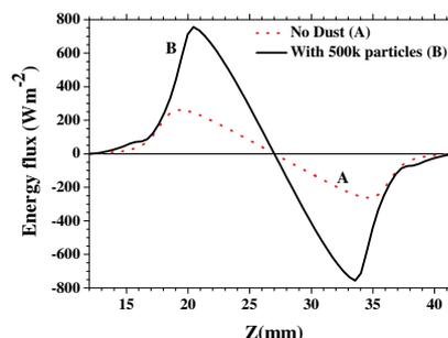
Figure 4:  $\Gamma_w$  along the central axis of the discharge, between the electrodes.
