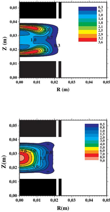
Figure 3: Energy taken up by electrons ( $\text{kW m}^{-3}$ ) (top) and ionization rate ( $\times 10^{20} \text{m}^{-3} \text{s}^{-1}$ ) (bottom).
