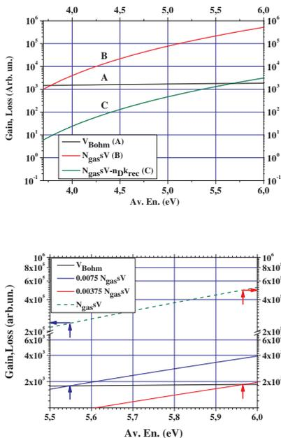
Figure 1: Particle balances. Dust as volume loss (top) and surface loss (bottom).
