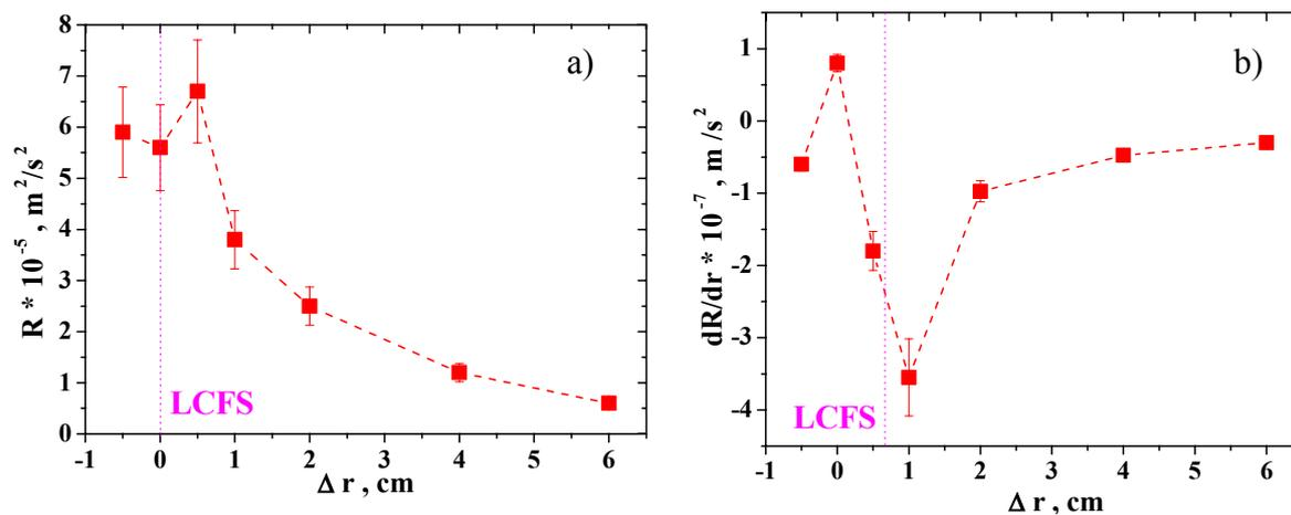
Fig. 3. Radial profiles of Reynolds stress component  $R$  (a) and  $dR/dr$  (b).
