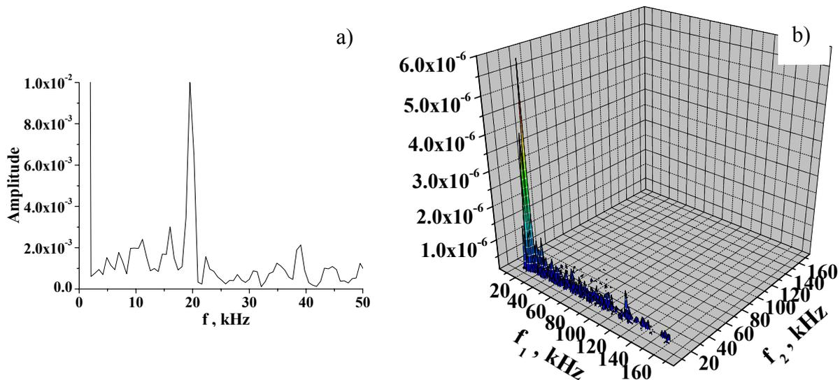
Fig. 1. Power spectrum (a) and bispectrum (b) of the floating potential fluctuations at the LCFS.
