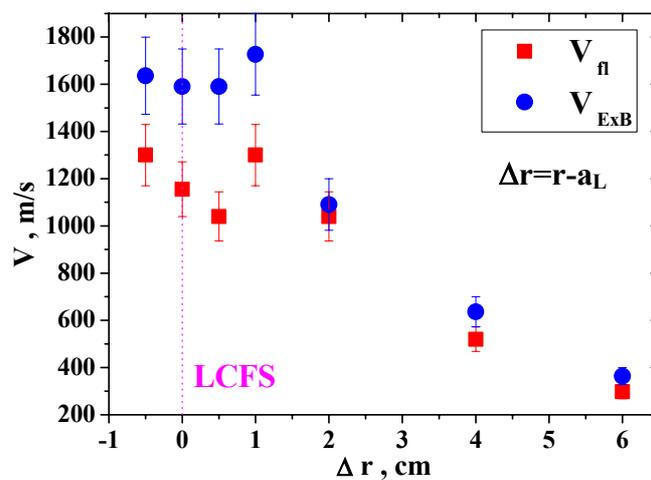
Fig. 2. Radial profiles of poloidal phase velocity ( $V_\pi$ ) and poloidal electrical drift velocity ( $V_{ExB}$ ).
