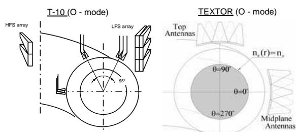
Fig. 1. Positions of correlation reflectometer antennae arrays in T-10 (left) and TEXTOR (right).
