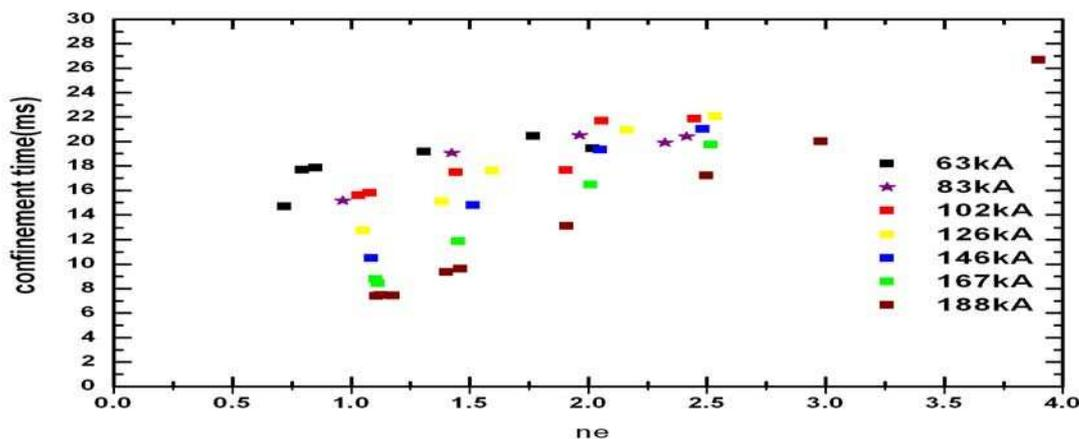
Fig.1. Energy confinement time with various electron density and current
