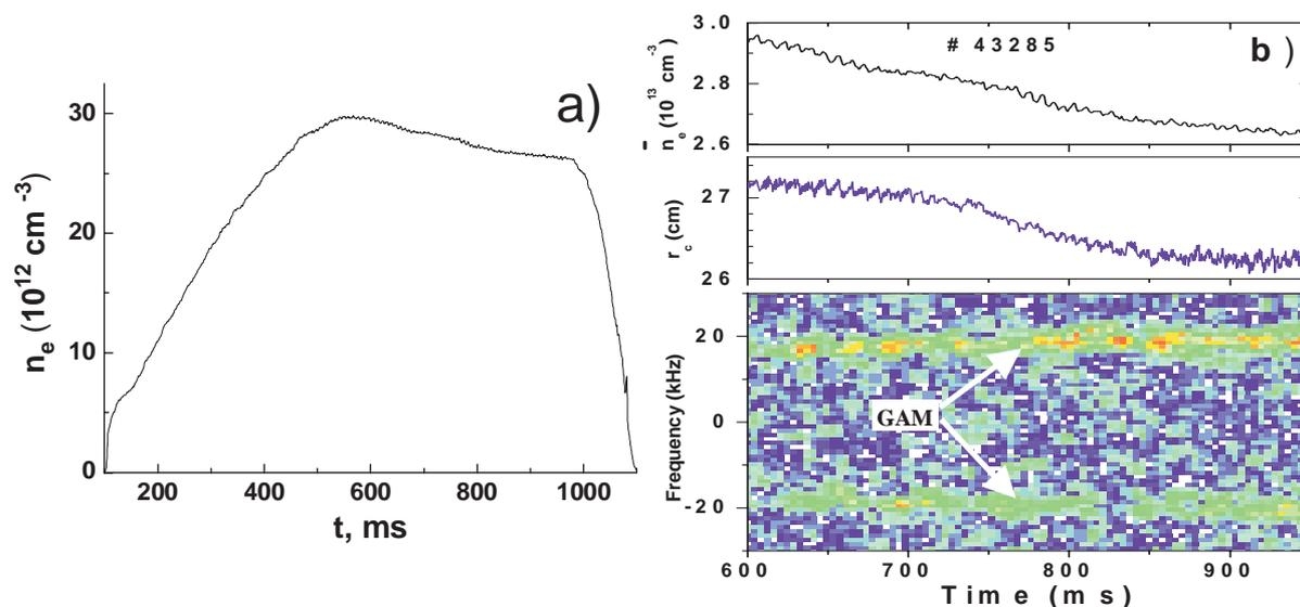
Fig. 5. Radial evolution of the long-distance potential-density correlations. a) Time trace of the density evolution in the OH discharge. b) Potential-density correlation for different radii for one shot. HIBP versus CR. Top box- line average density evolution. Middle box – corresponding CR observation radius. Bottom box - potential-density correlation coefficient. HIBP radial position is  $r = 25 \pm 0.5$  cm.
