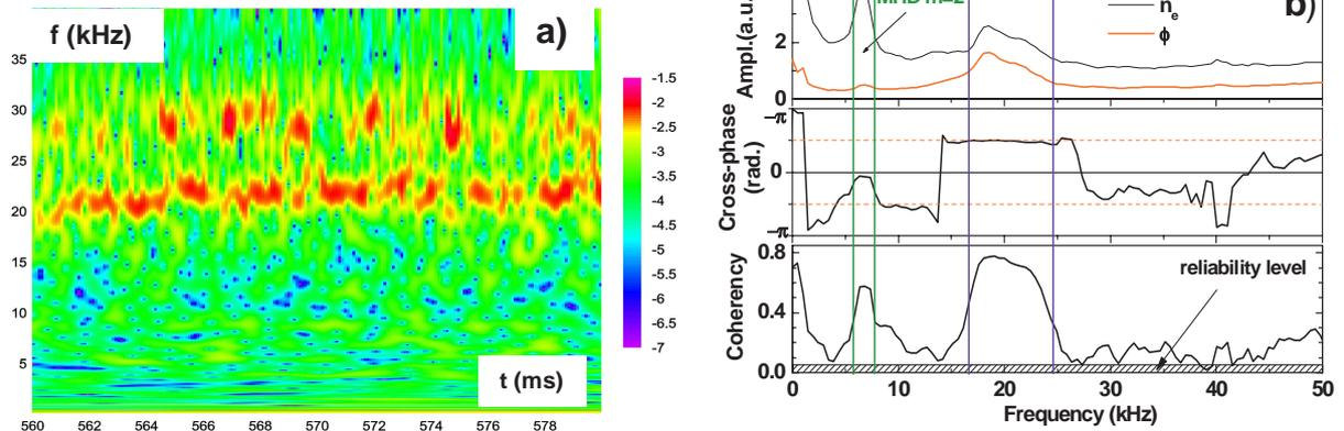
Fig. 2. a) Wavelet spectrogram for HIBP potential. ECR heated plasma. b) Local potential-density correlation. HIBP shows that GAM oscillations are more pronounced on the potential than on the density. In contrast, the amplitude of 7 kHz MHD  $m=2$  oscillations is larger on the density and much smaller on the potential.
