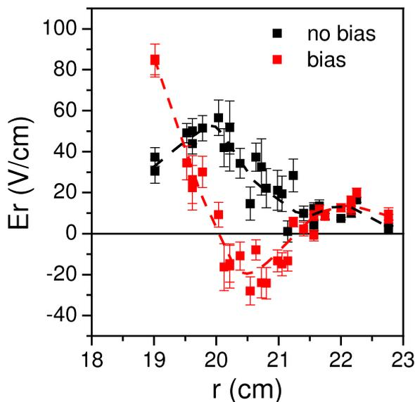
Figure 4. Radial electric field in the SOL measured by the rake probe
