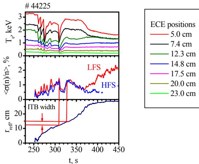
Fig. 3 Temperature evolution measured by ECE diagnostics from different chords, turbulence amplitude measured at Low and High Field Side, position of reflection layer (at LFS) for the typical shot with ITB formation.
