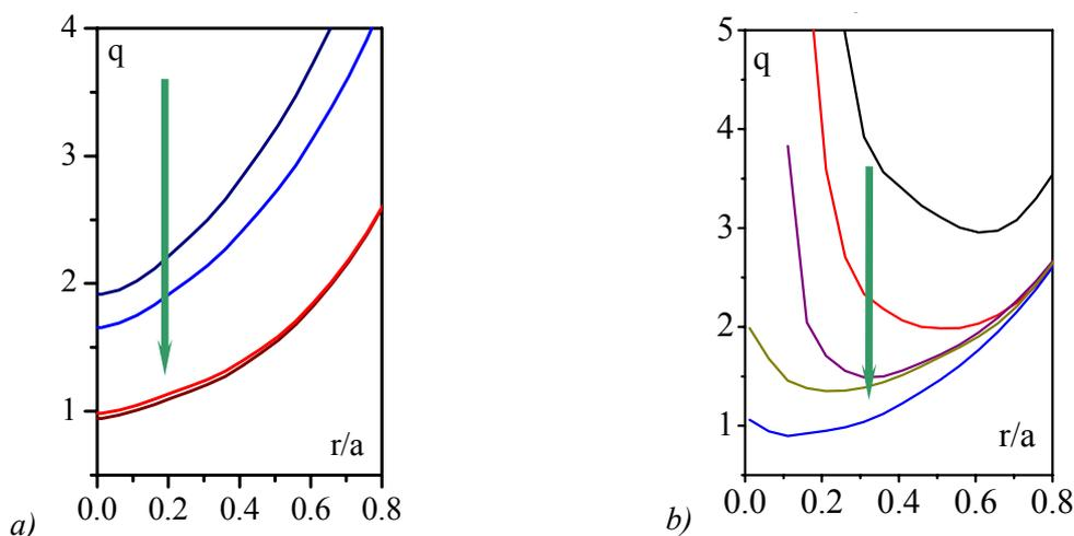
Fig. 5 Difference in  $q(r)$  profile evolution in ohmic discharge (a) and in discharge with early ECRH application,  $P_{ECRH}=0.95$  MW (b). Direction of changes with the time is shown by arrows.
