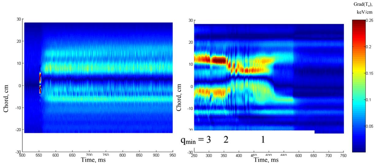
Fig. 2 Evolution of the temperature gradient in usual T-10 L-mode (left), i.e. monotonous  $q(r)$  profile, and in ITB case (right). Global discharge parameters and heating power value are the same in both cases. ECRH power has been applied at  $t = 550$  ms in L-mode case and at  $t = 200$  ms (together with  $I_p$  switch-on) in ITB case presented on this figure.
