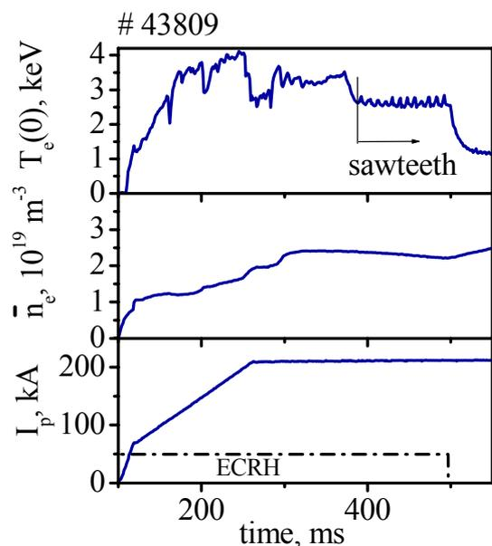
Fig. 1 Typical scenario of T-10 discharge with reversed shear and ITB formation.
