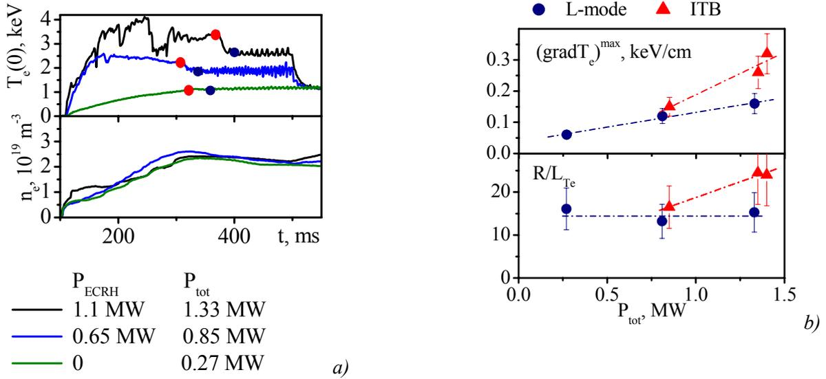
Fig. 4 (a) typical shots for investigation of power dependence of ITB characteristics. Typical instants for comparison between L-mode and ITB are shown by coloured circles; (b) dependence of ITB characteristics on total heating power in comparison with the L-mode.
