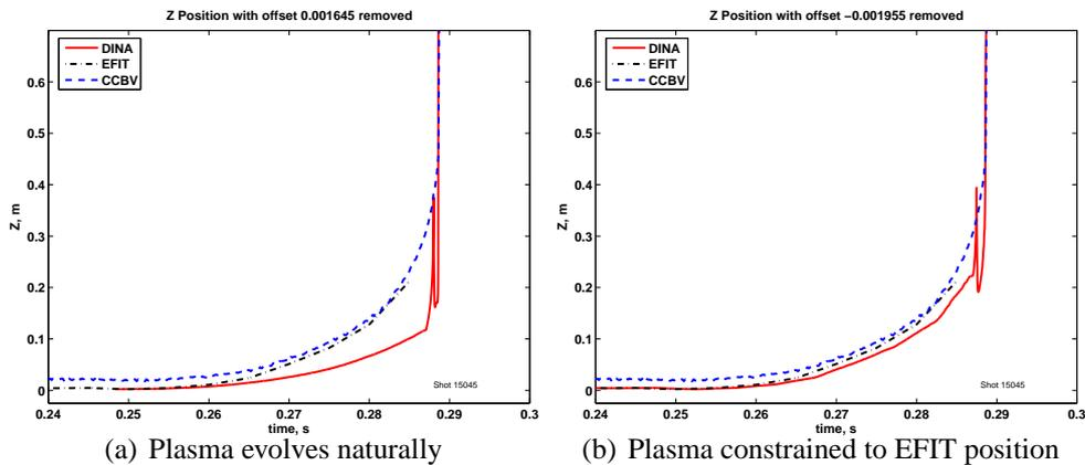
**Figure 2:** Evolution of the plasma vertical position during the VDE.
