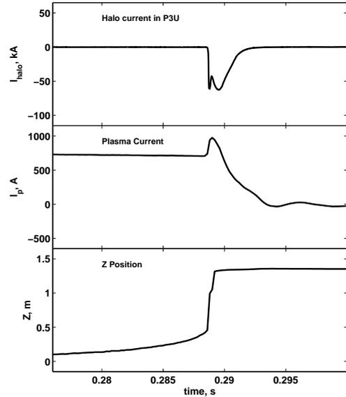
**Figure 1:** Halo currents in the upper P3 leg, plasma current and plasma Z position for shot 15045.
