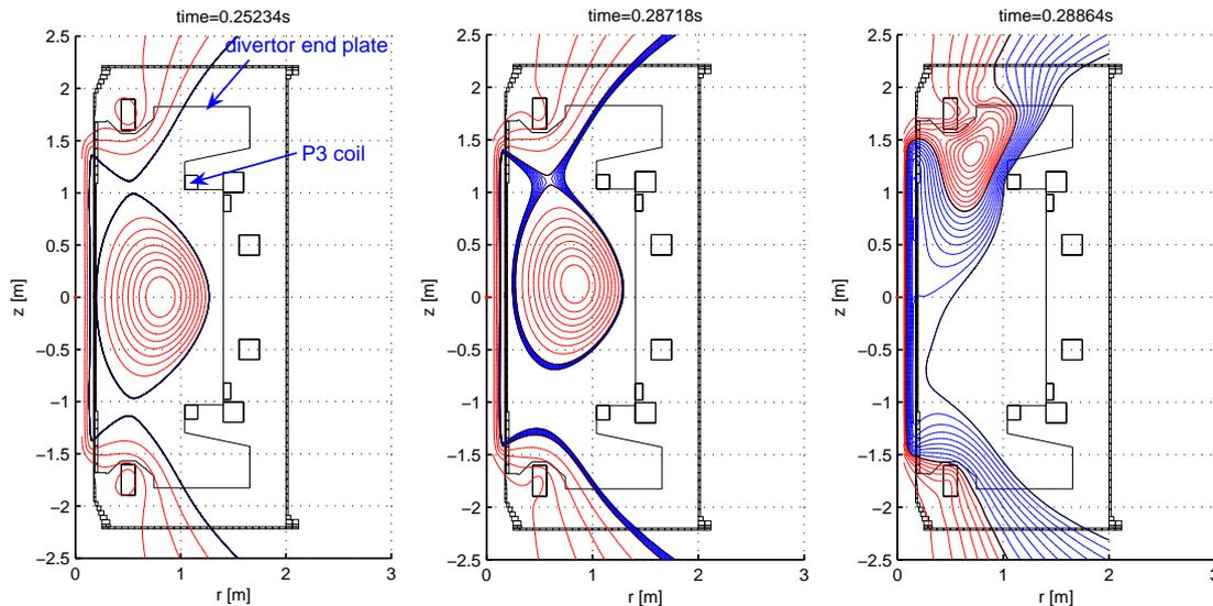
**Figure 3:** Poloidal cross-section of the MAST vessel showing the halo region in blue and the black boundary line depicting the plasma-facing surfaces (simplified) with which the plasma or halo region could come into contact.
