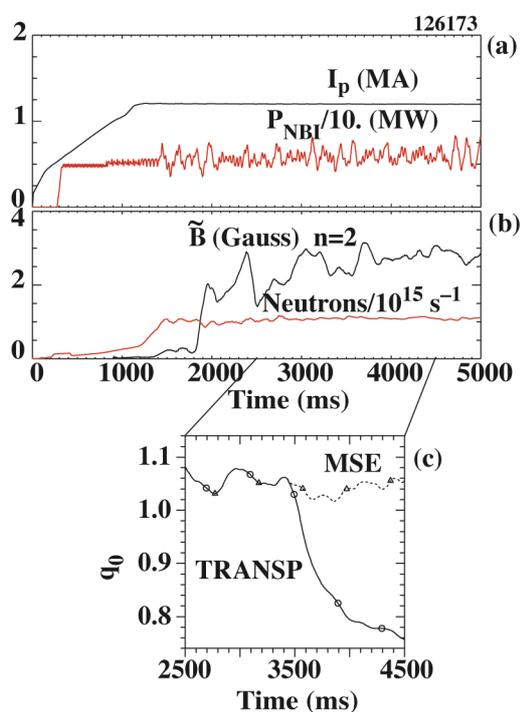
Fig. 1. Time evolution of plasma parameters for hybrid discharge 126173: (a) plasma current and beam power, (b) rms mode amplitude for  $m/n=3/2$  mode and neutron rate, (c) evolution of  $q(0)$  from MSE and TRANSP without MSE after 3.5 s. Plasma parameters are:  $B_T=1.8$  T,  $I_p=1.2$  MA,  $R_0=175$  cm,  $T_e(0) \approx 3.2$  keV,  $n_e(0) \approx 5 \times 10^{13} \text{ cm}^{-3}$ .
