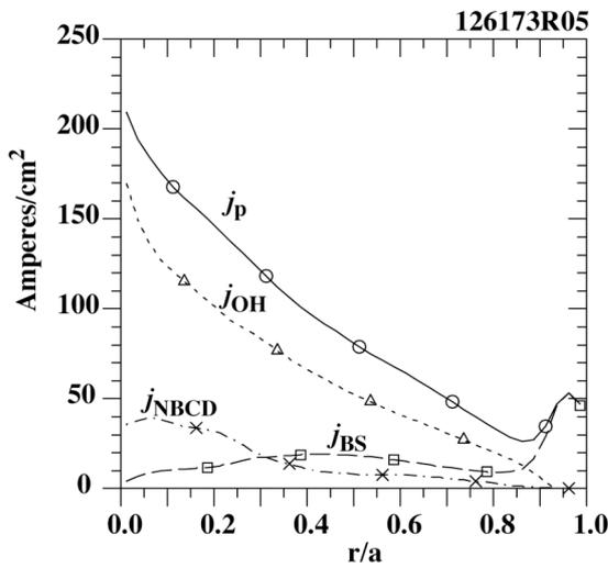
Fig. 3. Current density profiles vs normalized minor radius from TRANSP for 126173 at 4.5 s. Plasma current ( $j_p$ ), Ohmic current ( $j_{\text{OH}}$ ), neutral beam current ( $j_{\text{NBCD}}$ ), bootstrap current ( $j_{\text{BS}}$ ).
