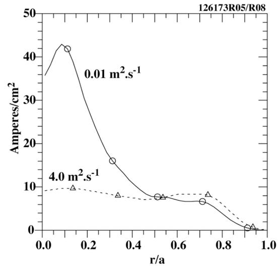
Fig. 4. Beam driven current density profiles from TRANSP for  $D_{\text{fast}}=0.01 \text{ m}^2 \cdot \text{s}^{-1}$  and  $D_{\text{fast}}=4.0 \text{ m}^2 \cdot \text{s}^{-1}$ . The enhanced diffusivity extends to 0.7 minor radius.
