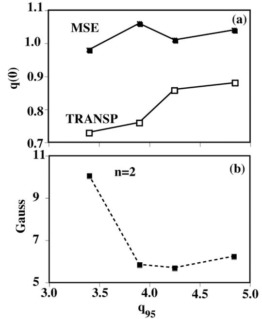
Fig. 2. (a) Measured  $q(0)$  from MSE and simulated  $q(0)$  from TRANSP at 4.5 s. into the discharge vs  $q_{95}$  for a reproducible set of hybrid discharges with a strong  $m/n=3/2$  mode. (b) Estimate of the  $n=2$  RMS poloidal magnetic field at the  $q=3/2$  surface.
