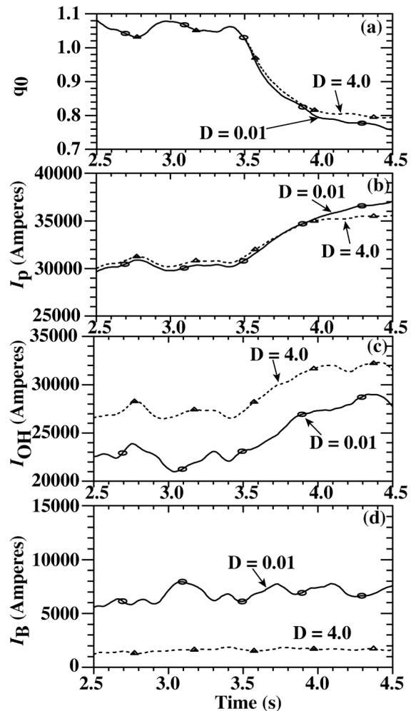
Fig. 5. Time evolution from TRANSP for  $q(0)$  (a) and plasma current inside  $r/a=0.1$ :  $I_p$  (b)  $I_{OH}$ , (c)  $I_{NBCD}$  (d).  $D_{fast}=0.01 \text{ m}^2.\text{s}^{-1}$  (solid) and  $D_{fast}=4.0 \text{ m}^2.\text{s}^{-1}$  (dashed). The TRANSP loop voltage increases from the measured 0.11 V at 3.5 s to 0.16 V by 4.5 s.
