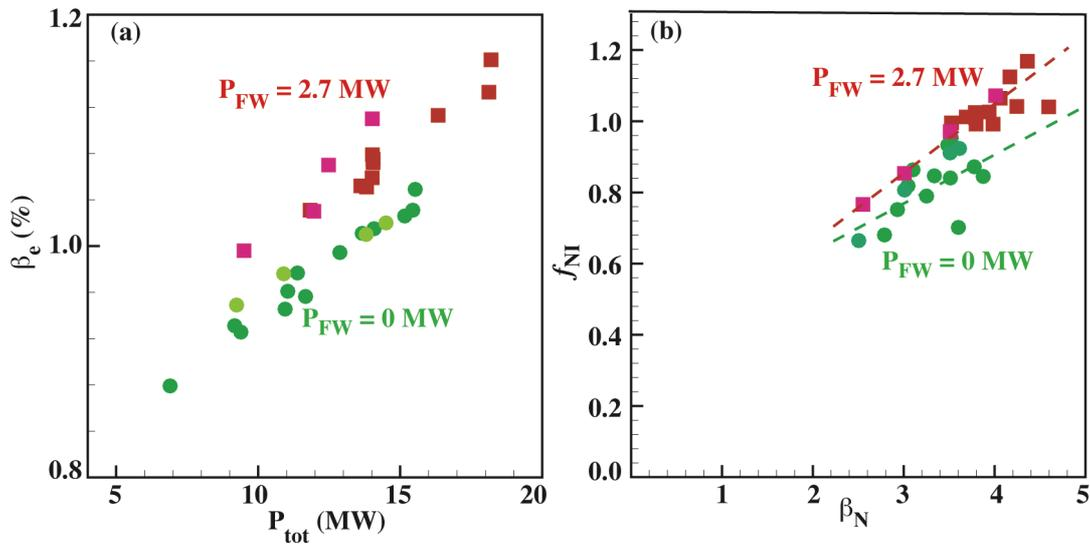
Fig. 2. (a) Electron beta and (b) noninductive current fraction as a function of (a) total heating power and (b) normalized beta for two different fast wave heating power,  $P_{FW} = 0$  MW (circles) and  $P_{FW} = 2.7$  MW (squares), in the ONETWO/GLF23 simulation database.
