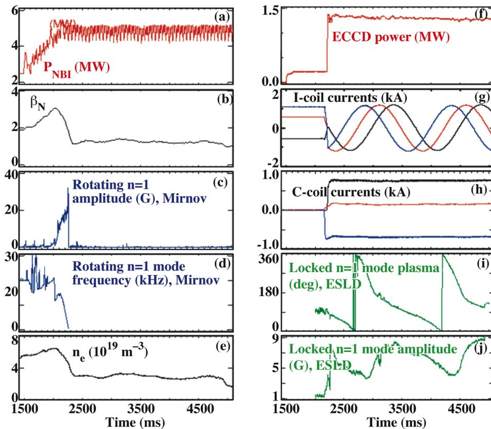
Fig. 1. Evolution of (a) NBI power, (b)  $\beta_N$ , (c) rotating  $n=1$  growth rate and (d) frequency, (e) density, (f) ECCD power, (g) I-coil and (h) C-coil currents, (i) phase and (j) radial field amplitude of locked  $n=1$  mode. #126623.
