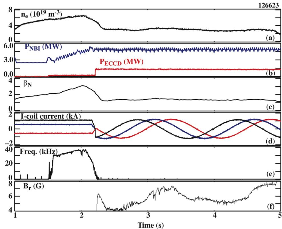
FIG. 3. Evolution of (a) density, (b) neutral beam and electron cyclotron current drive power, (c)  $\beta_N$ , (d) I-coil currents, (e) NTM mode frequency, and (f) radial magnetic field due to the magnetic island. Prior to 2.2 s, I-coil current is applied for error field control.
