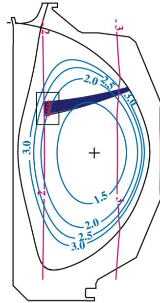
FIG. 1. (a) Cross-section of the DIII-D discharge showing the rational  $q$  surfaces. The rays of the EC beam are shown as the blue lines, and the magenta lines marked 2 and 3 are the second and third harmonics of the electron cyclotron resonance. Rational  $q$ -surfaces are shown.
