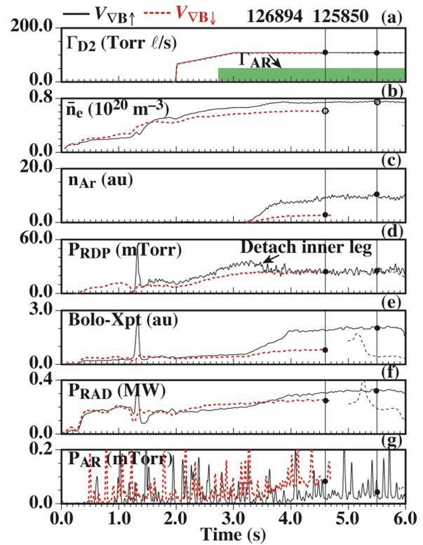
Fig. 2. Two upper SN ( $drsep = +1.0$  cm) H-mode discharges with opposite  $\mathbf{B} \times \nabla B$  direction,  $V_{\nabla B\uparrow}$  (solid) and  $V_{\nabla B\downarrow}$  (dashed), are compared. “Steady-state” timeslices are denoted by the vertical lines.
