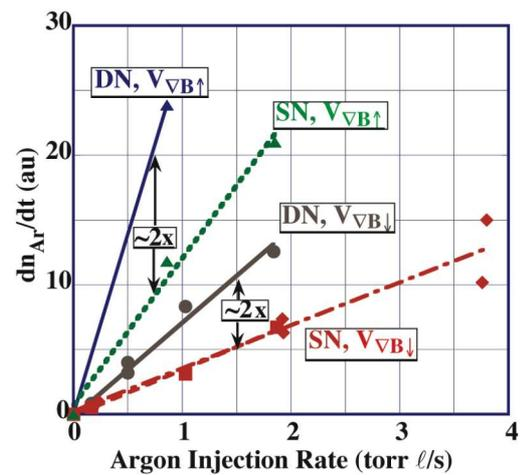
Fig. 5. The initial rate of argon accumulation in SN and DN plasmas is plotted versus  $\Gamma_{AR}$  for both  $V_{VB\downarrow}$  and  $V_{VB\uparrow}$  cases.
