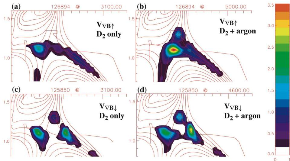
Fig. 3. Tomographic inversions of bolometric arrays are shown for SNs with  $V_{\nabla B\uparrow}$  (a) with deuterium injection only and (b) deuterium and Ar injection together. Also shown are inversions for SNs with  $V_{\nabla B\downarrow}$  (c) deuterium injection only and (d) deuterium and Ar injection together. Only the upper divertor region is shown.
