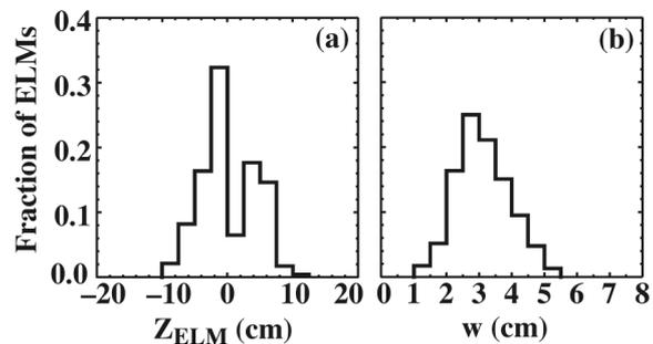
Figure 3. Distributions of (a) location  $Z_{ELM}$  where ELM filaments hit the outer wall, and (b) poloidal filament width  $w$ .
