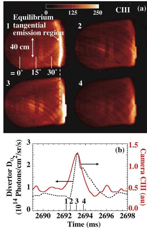
Fig. 1. (a) Images in CIII light of an ELM-driven plasma show multiple field-aligned filaments are ejected into the SOL. (b) The integrated camera intensity is compared to the inner divertor  $D_\alpha$  signal, and the times of images 1–4 are labeled.
