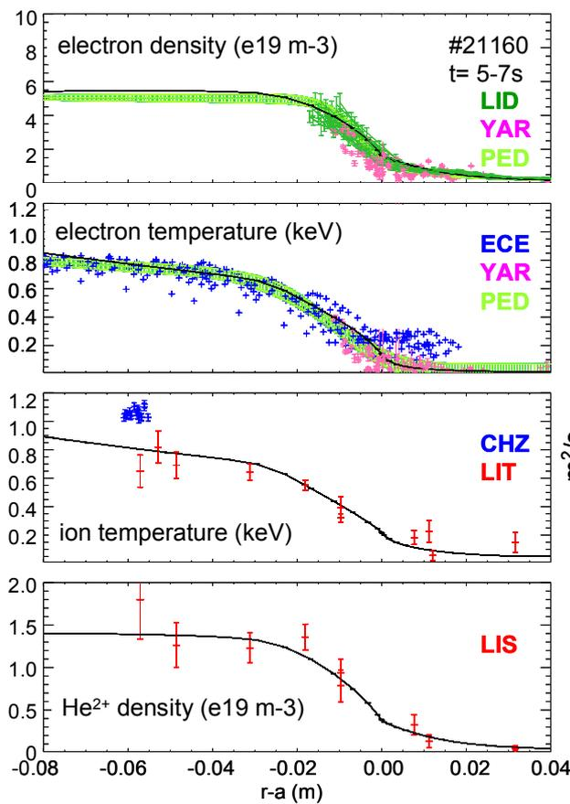
Figure 3 (left): Mid-plane profiles from various diagnostics (symbols: LID = Lithium beam, YAR= Thomson scattering, ECE = electron cyclotron emission, CHZ = core charge exchange, LIT = Li-beam CXRS, LIS = Li-beam CXRS, PED = ‘tanh’ fit to  $n_e$  and  $T_e$  profiles) in comparison with the model (black lines).
