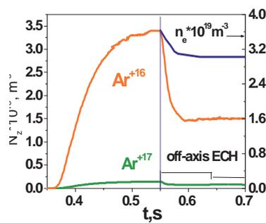
Fig.5.Simulated Ar ions and electron densities evolution in OH regime and after off-axis ECH switch on.
