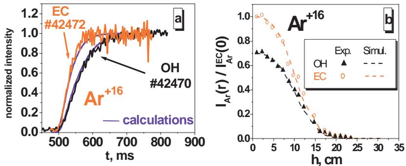
for transport calculations are given in Fig.2. (a) and (b). Fig.2a shows evolution of the central chord line radiation in OH and on-axis ECH regimes after Ar puffing. Ar<sup>+16</sup> chord radiation profiles in steady-state are shown in Fig.2b.
