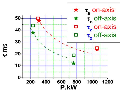
Fig.7 Energy confinement times and impurity confinement times (decay times) versus the total power. ---- ITER scaling L- mode  $\tau_E \sim 1/P^{0.73}$
