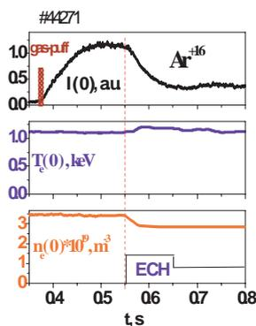
Fig.4. Measured time traces of  $Ar^{+16}$  chord line radiation,  $n_e$ ,  $T_e$
