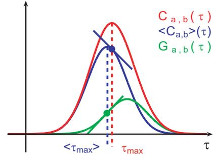
Figure 3: The effect of 'difference'-function on the displacement of the CCF maximum.
