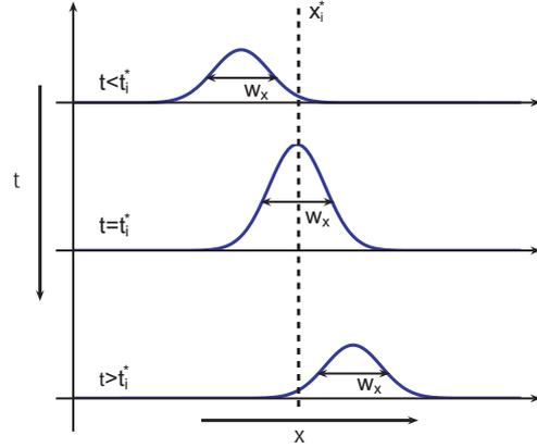
Figure 1: Illustration of propagating Gauss-shaped structures
