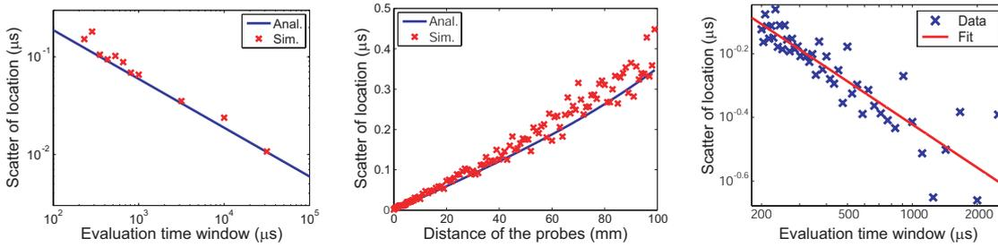
Figure 4: Analytic (blue line) and simulated (red cross) dependence of the uncertainty of the time shift on the length of the evaluation time window and probe distance: left and middle. Dependence of the uncertainty of the time shift on the length of the evaluation time window in measured data (blue cross) and the fitted function (red line): right.
