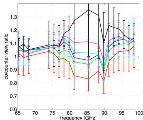
Fig. 3 The ratio of the co-/counter-viewing receiver signals as a function of frequency. The driven current is increased from counter- to co-ECCD (red to black curves). The central frequencies (81.25 – 88.34 GHz) are from the region of current generation. The EDF is seen to be asymmetric and emits more radiation in the direction of driven current.
