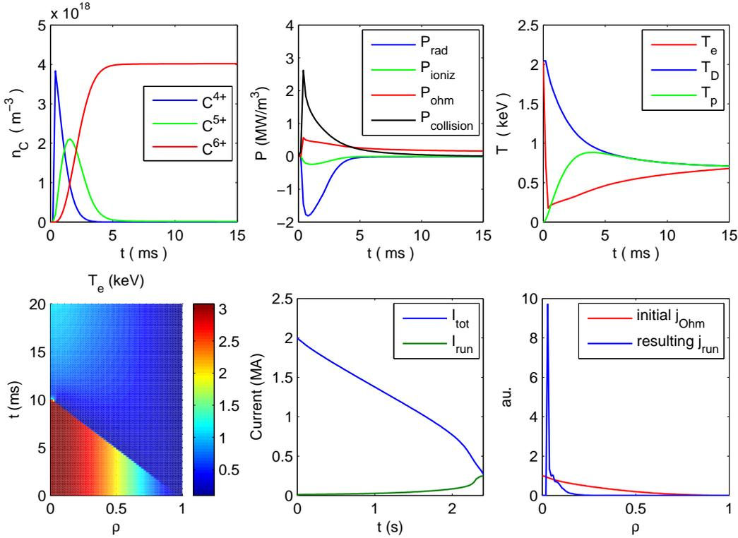
Figure 1: Simulation of a  $v_p = 100$  m/s,  $r_p = 0.9$  mm carbon pellet, with  $\chi = 1$  m<sup>2</sup>/s. Top plots show  $\rho = r/a = 0.5$ : Left: Carbon ionisation. Middle: Electron energy loss and gain. Right: Temperatures of electrons, deuterons and pellet ions. Bottom: Left: Electron temperature. Middle: Ohmic and runaway currents. Right: Current densities.
