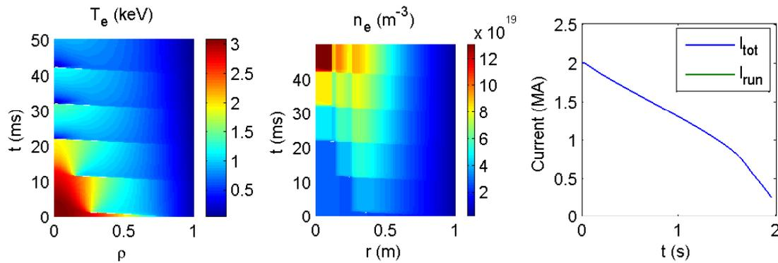
Figure 2: Multiple  $v_p = 500$  m/s,  $r_p = 0.6$  mm carbon pellets. Left: Electron temperature. Middle: Thermal electron density. Right: Ohmic current.
