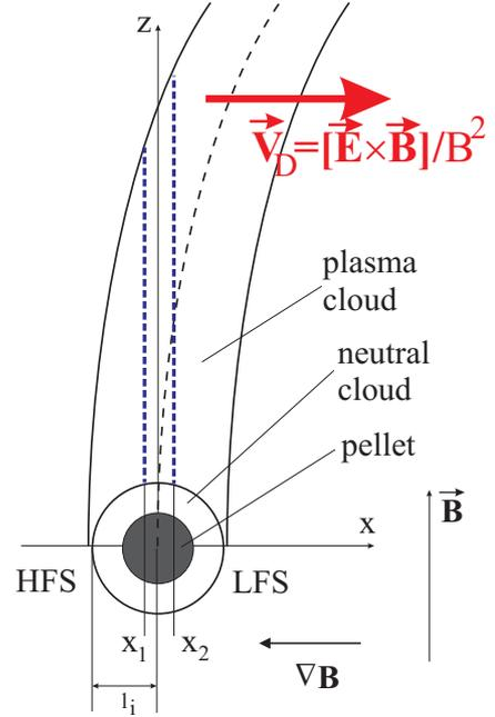
Figure 2. Cross-section of drifting cloud by  $xz$ -plane. Blue dash lines show plasma cloud thickness at different  $x$ .
