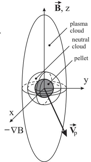
Figure 1. Scheme of pellet ablation cloud.
