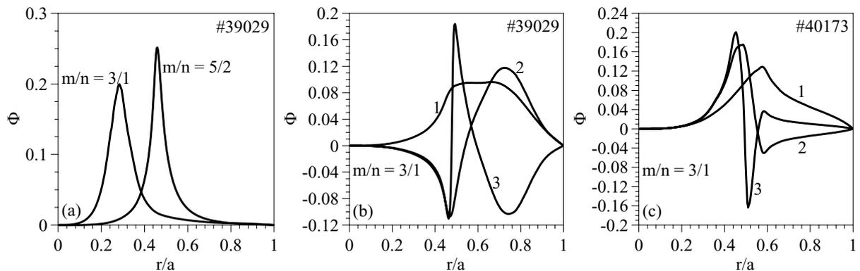
Fig. 1. Calculated AEs in the W7-AS shots #39029 and #40173: (a) GAE in AIs with the lowest frequency (33 kHz) and highest frequency (46kHz), respectively, in the shot #39029; (b) NGAE in AIs with intermediate frequencies of the shot #39029; curve 1, AI with the frequency of 38 kHz; curve 3, 35 kHz; (c) NGAEs relevant to AI in the shot #40173.
