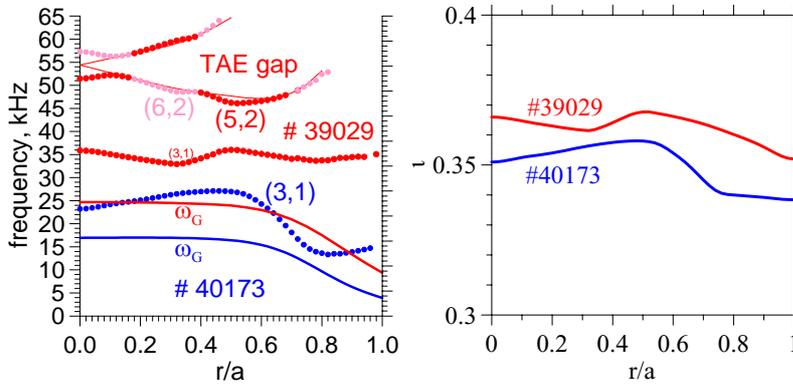
Fig. 2. Continuum branches with given  $(m,n)$  and the geodesic frequency,  $\omega_G$ .
