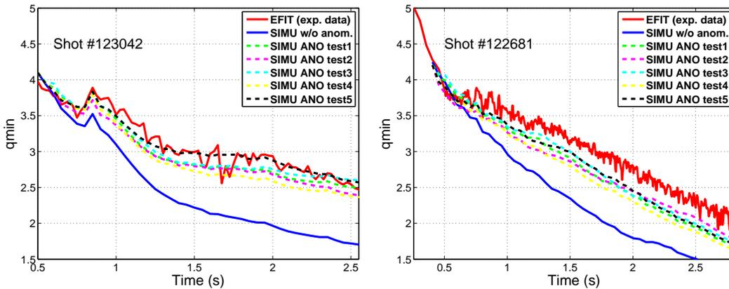
Figure 3:  $q_{min}$  time evolution for shots #123042 and #122681, as measured by EFIT and simulated by CRONOS, first without fast ion anomalous transport, then with the five sets of anomalous transport coefficients tested.
