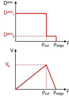
Figure 1: *Simplified shape of the ad-hoc diffusion coefficient and convection velocity profiles.*
