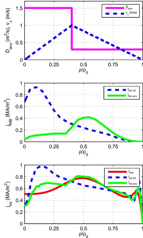
Figure 5: Profiles of diffusion coefficient and convection velocity fitting the experimental  $q_{\min}$  evolution (i.e. test 5), and associated NBI and total current profiles, for shot #123042 at  $t=2\text{s}$ .
