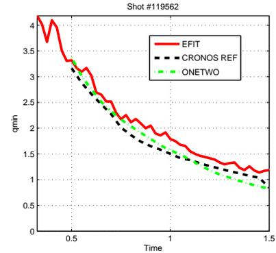
Figure 2: *CRONOS and ONETWO simulations of the minimum safety factor  $q_{\text{min}}$  evolution compared to the experiment for shot #119562.*
