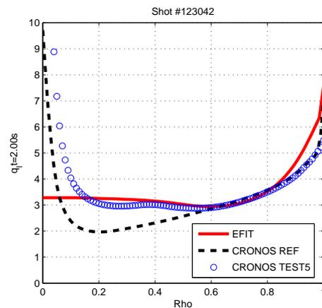
Figure 4: Experimental and simulated  $q$ -profiles for shot #123042 at  $t=2s$ .
