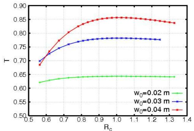
Figure 5: Dependence of  $T$  on the matching parameter  $R_c \equiv R_p/R_b$ , for different beam waists.
