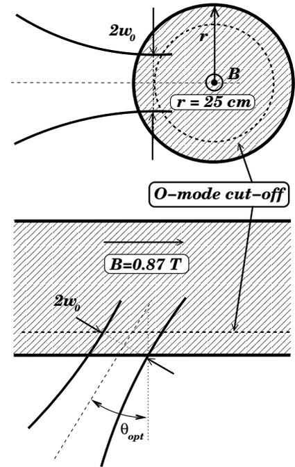
Figure 3: Cylindrical plasma used in the 2–D full wave calculations.  $R_p \equiv r = 25$  cm.
