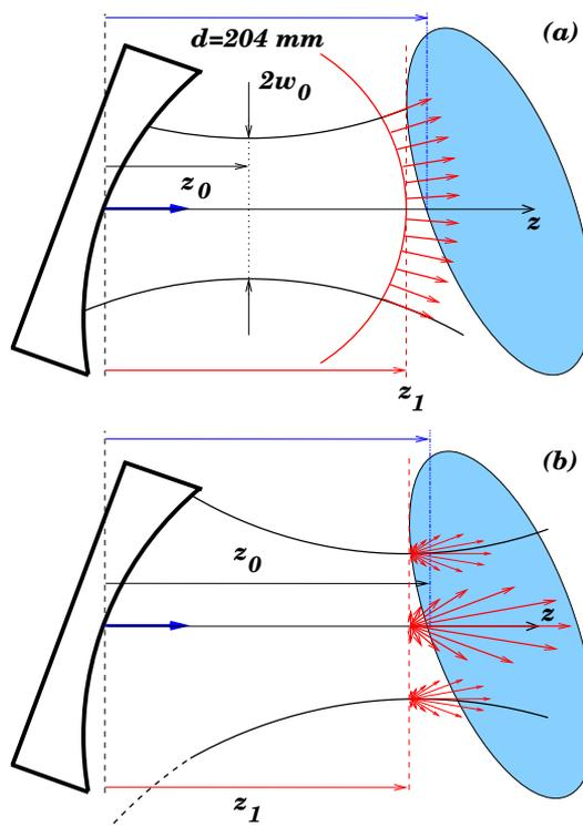
Figure 1: *Schematic beam representation. (a) Perpendicular rays distribution for any  $z_0$  and (b) plane wave spectrum distribution used for  $z_0 = 0.2$  m.*
