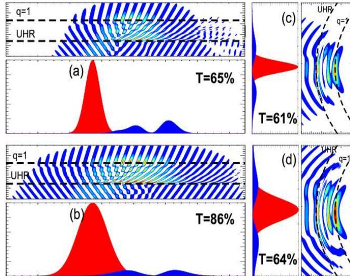
Figure 4: Full–wave calculations in the horizontal (left) and vertical (right) planes. The conversion efficiency  $T$  is shown in the graphs. The reflected power is due to the unconverted power–fraction from the wings of the angular beam pattern.
