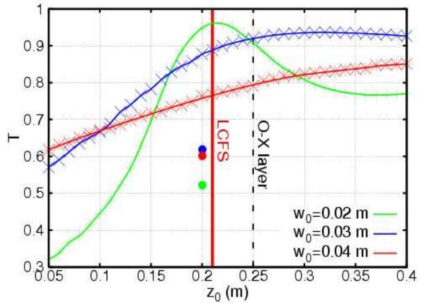
Figure 2: Total conversion efficiency obtained in the TJ-II stellarator ( $\omega/2\pi = 28$  GHz) with the perpendicular rays approximation (solid lines) and the  $\mathbf{k}$  spectrum approach (dots). The O-X layer and the LCFS location are shown.
