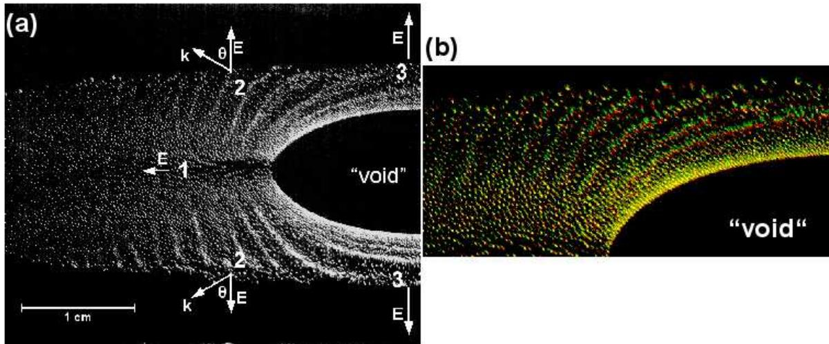
Fig. 2: (a) Vertical section through the dust cloud. Self-excited dust density waves emerge at the void edge and propagate into the dust cloud. (b) Closeup of the upper left quadrant of the dust cloud. The image is a superposition of two successive video frames (frame 1: red, frame 2: green).
