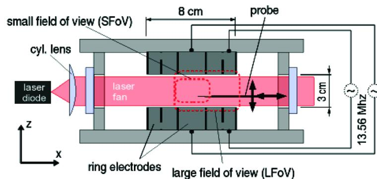
Figure 1: Vertical section through the IMPK-K discharge chamber. From [1].
