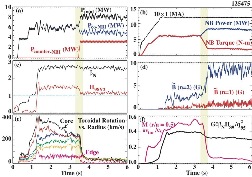
Fig. 1. Hybrid discharge quality  $\{\beta_N, H_{98Y2}, G\}$  is maintained as core toroidal rotation (e) is decreased from  $M=0.5$  to  $M \sim 0.1$  (f) with counter neutral beam injection (a,b). A slight reduction in  $H_{98Y2}$  results in a 20% reduction in  $G$ . The benign  $n=3/2$  MHD mode suppresses sawteeth, and increases as the rotation decreases (d).
