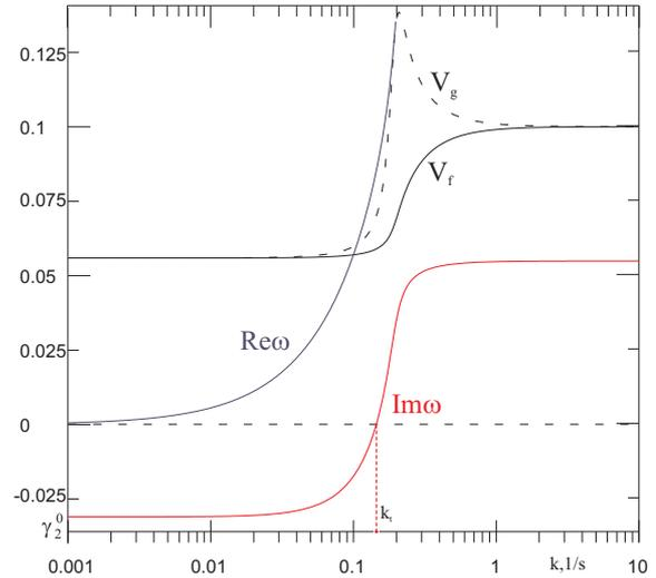
Figure 3: SIC instability dispersion curves,  $N_q = 0.6 \text{ cm}^{-3}$ ,  $R = .015 \text{ cm}$ ,  $f_N = 0.173 \text{ s}^{-1}$ ,  $v_i = 0.039 \text{ s}^{-1}$
