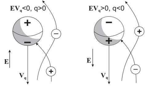
Figure 1: Selective ion capture charging for a single particle.
