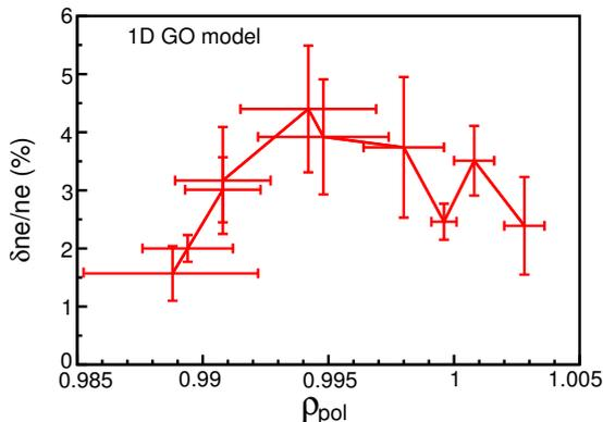
Figure 4: Density fluctuation level profile using 1D Geometric Optics model for shot #20354.
