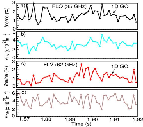
Figure 3: Temporal evolution of (a) density fluctuation level deduced from Q band reflectometer signal, (b) its associated  $\nabla n_e$ , (c) density fluctuation level from V band reflectometer signal and (d) its associated  $\nabla n_e$  for shot #20393.
