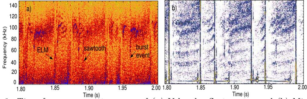
Figure 2: Time-frequency spectrograms of (a) V band reflectometer and (b) Mirnov coil signals for shot #20393.
