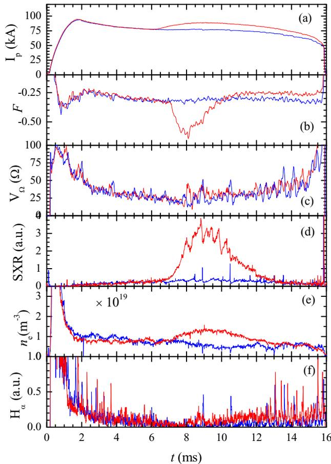
Figure 5. Reference discharge (blue, #20989) and aided PPCD without FB (red, #20993): reference (a) plasma current, (b) reversal parameter, (c) resistive loop voltage, (d) SXR signal, (e) electron density and (f)  $H_{\alpha}$  signal.
