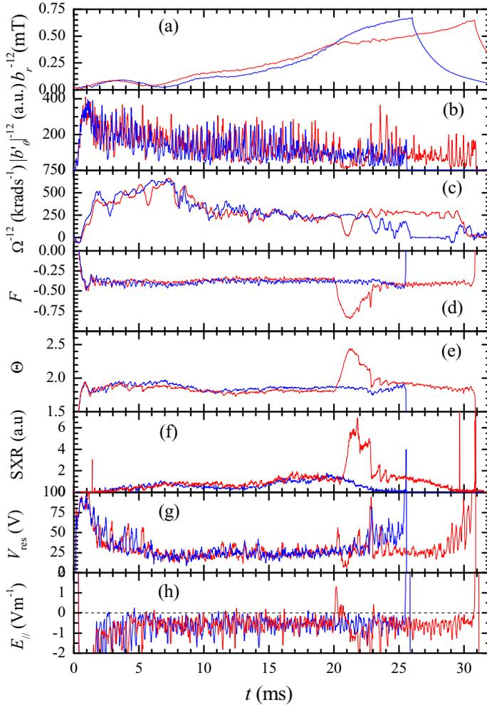
Figure 1. Time evolution of the global parameters for discharges with selective AFS only (blue, #20892) and with the addition of PPCD (red, #20900). From top to bottom: (a) radial component of TM  $n = -12$ , (b) poloidal component of TM  $n = -12$ , (c) helical phase velocity (d) reversal parameter, (e) pinch parameter, (f) SXR, (g) resistive loop voltage and (h) parallel electric field.
