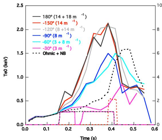
**Fig. 1** Central electron heating in D plasma as a function of array phase shift. 1.1 MW HHFW applied from 0.15-0.41 s (RF trip at 0.23 s for  $-30^\circ$  phase). 2 MW NBI from 0.38-0.42 s.
