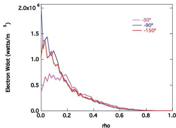
**Fig. 6** AORSA electron power deposition profiles for 128662 show less centrally peaked heating for the  $-30^\circ$  case. This case also shows some ICH minority heating ( $\sim$ 2% of total power).
