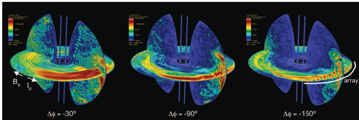
**Fig. 5** AORSA E-fields for shot 128662 (1.1 MW, Te(0)  $\sim$  1.5 keV, Ti (0)  $\sim$  800 eV, D with 2% H) for three array phasings
