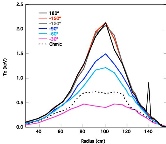
**Fig. 3** Electron temperature profiles at 0.38 s shows increased heating at larger phase shifts ( $k_{\parallel}$  predominantly  $14 \text{ m}^{-1}$ )
