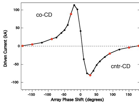
**Fig. 7** In the absence of plasma edge losses, AORSA predicts CD efficiency for the Te(0)  $\sim$  1.5 keV plasma to be most efficient for  $-30^\circ$ . (Red dots are attainable phasings for the 12-element array as configured).
