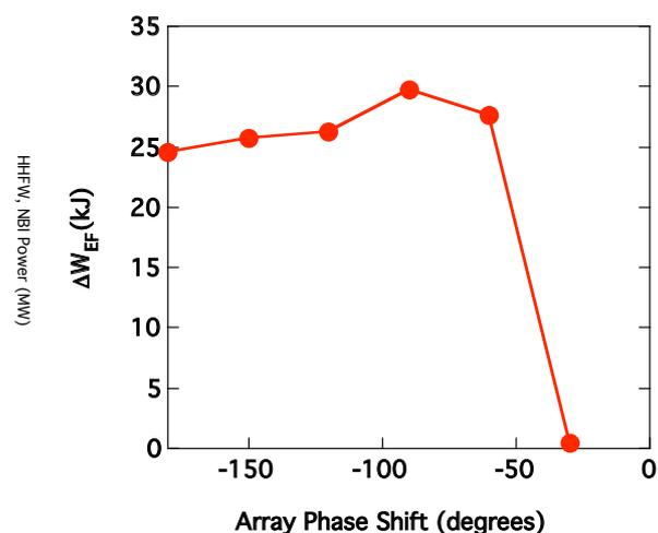
**Fig. 2** Change in total stored energy (EFIT calculation) at 0.38 s as a function of array phase shift for 1.1 MW HHFW. Heating efficiency stays fairly constant from  $-180^\circ$  to  $-60^\circ$ .
