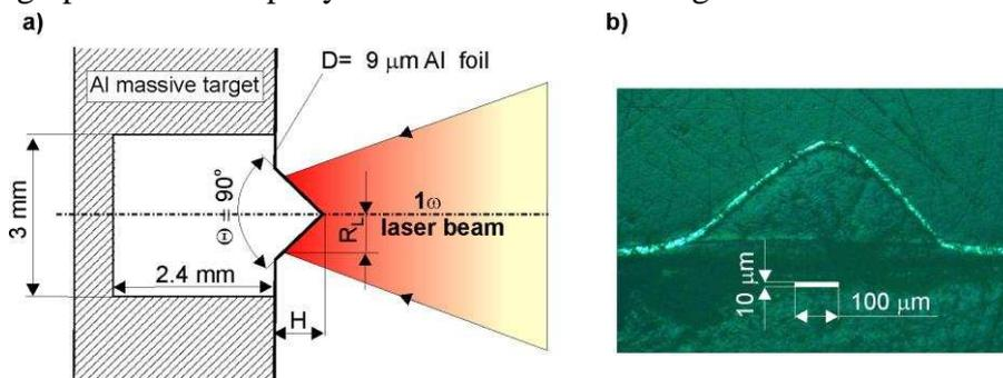
Fig. 4 The target construction (a) and the cross-section photograph of the exemplary Al cone (b).
