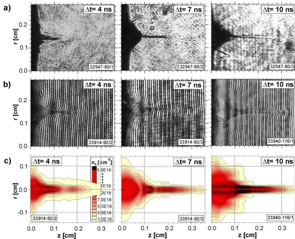
Fig. 1. Illustration of the typical plasma jet generated by the action of laser beam on the Cu planar target: a – shadowgrams, b – interferograms, and c – electron equidensitograms.
