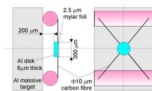
Fig. 2 Double target construction.
