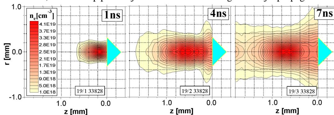
Fig. 5 Sequence of the electron equidensitograms corresponding to propagation of the cumulative jet.
