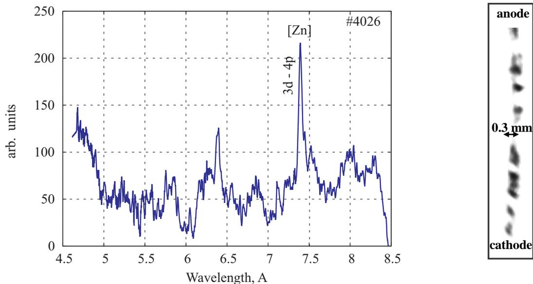
Fig 4. Spectrum of tungsten pinch in the photon energy range 1.5 - 2.5 keV obtained by the crystal spectrograph.
