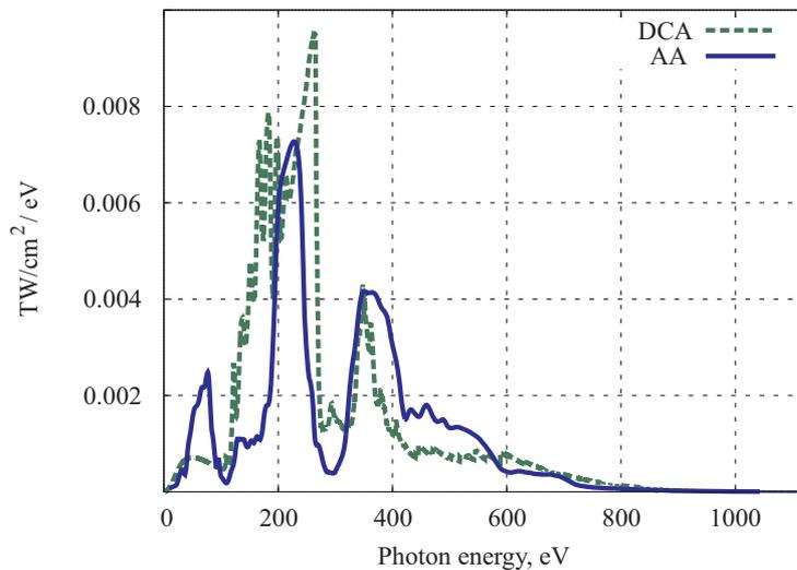
Fig.3. Comparison of the calculation results according to average atom model (AA) and detailed configuration accounting (DCA). Calculations were carried out for the electron density  $n_e = 10^{21} \text{ cm}^{-3}$  and temperature  $T_e = 75 \text{ eV}$ .
