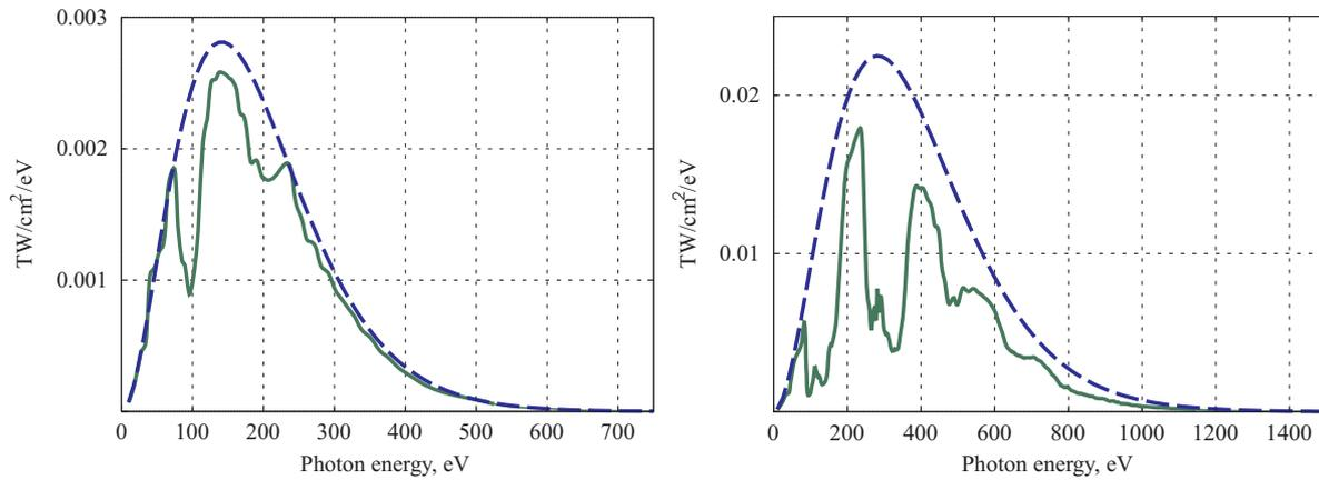
Fig.2. Simulation of Z-pinch spectra for a plane tungsten layer with electron density  $n_e = 10^{21} \text{ cm}^{-3}$  and different electron temperatures  $T_e$  (left -  $T_e = 50 \text{ eV}$ ; right -  $T_e = 100 \text{ eV}$ ). The Planckian at the corresponding temperature is shown by dashed line.
