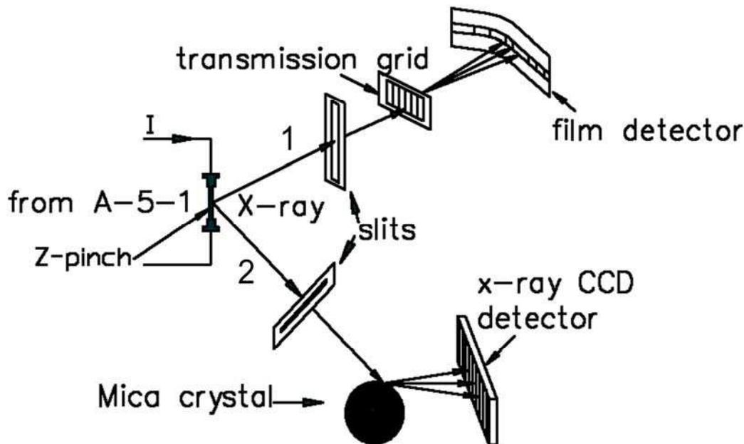
Fig.1. Experimental setup of Angara-5-1 spectral measurement diagnostics
