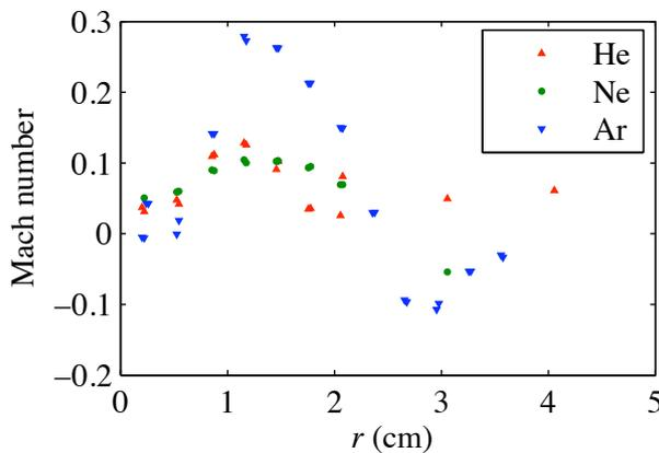
Figure 6. Radial profiles of Mach number
