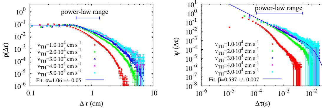
Figure 2: Step size pdf (left) and Waiting time pdf (right) for different  $v_{TH}$ . In both cases there exists a region where power-law decay is clearly detected, specially for  $v_{TH} = 3 \cdot 10^4$  cm/s.
