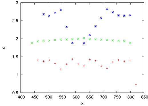
Figure 2: The safety factor profile along the minor radius for the initial state ( $\times$ , green), and in the SOC state for the standard threshold value ( $+$ , red), and for half the standard threshold ( $*$ , blue).
