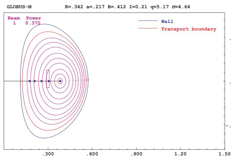
Figure 9. Equilibrium flux surfaces in H-mode. Bars show laser points, rectangle – the projection of NB. Lengths are in meters.
