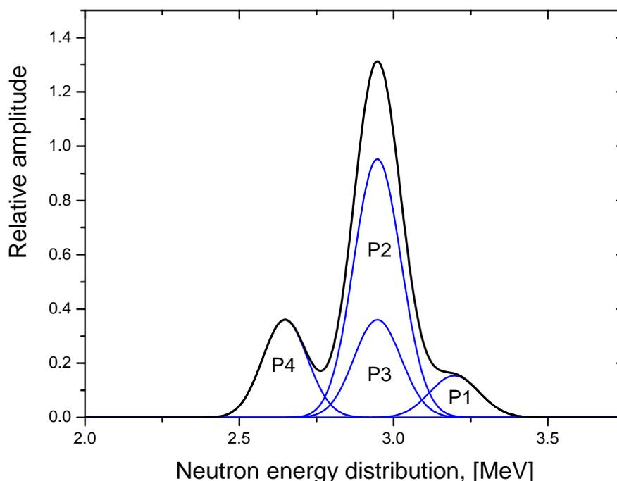
Fig. 2 Reconstructed energy distribution of the measured neutron TOF spectra.
