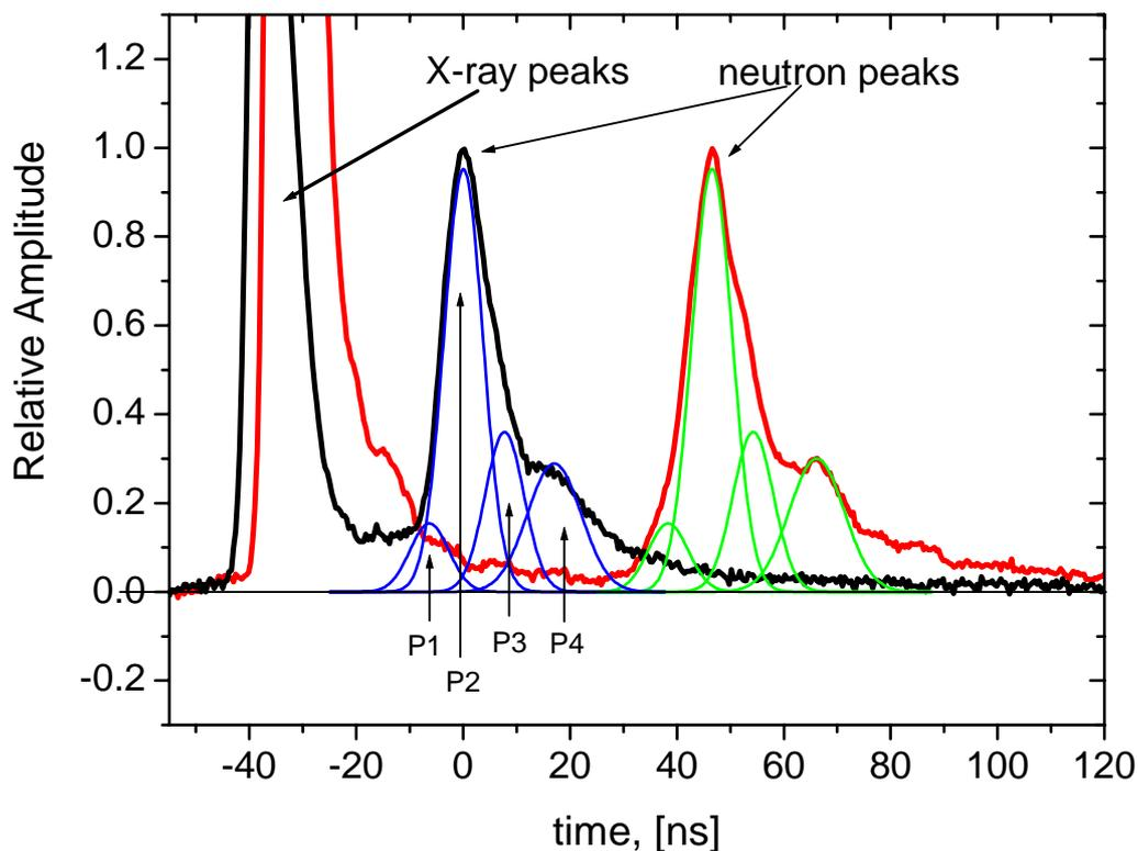
Fig. 1 Time-of-flight spectra measured at two different positions (black line -  $L_1=0.994\text{m}$ , red line -  $L_2=2.1\text{m}$ ); deconvoluted partial fluxes of neutrons.
