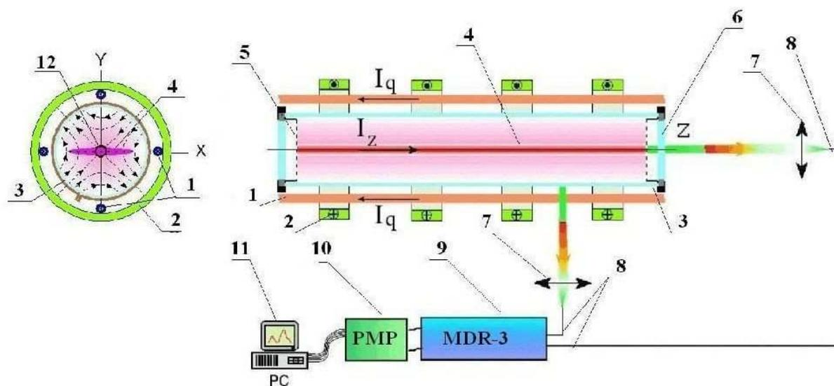
**Fig.1.** CS-3D device and diagnostics: (1) straight current conductors producing a 2D field, (2) coils producing a field  $B_z$ , (3) quartz vacuum chamber 18 cm in diameter and 100 cm long, (4) current sheet, (5) grid electrodes, (6) windows, (7) lenses, (8) quartz fibers, (9) monochromator, (10) photomultipliers, (12) plasma region under study.
