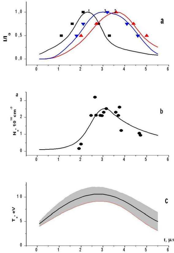
**Fig.2.** Measured (points) and calculated (curves) evolution of (a) spectral lines (1) Ar II 480.6 nm, (2) Ar III 379.5 nm, (3) C III 464.7 nm; (b) electron density  $N_e$ ; and (c) electron temperature  $T_e$ .
