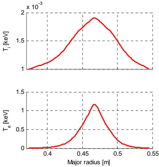
Figure 1. Ion (top) and electron (bottom) temperature profiles of ISTTOK.
