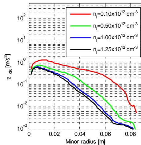
Figure 6. The kinetic ballooning contribution plotted for different electron density in ISTTOK.
