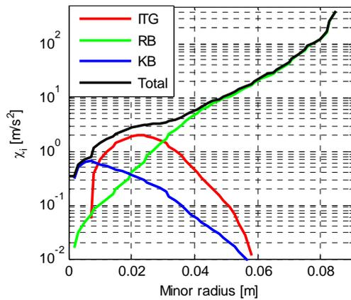
Figure 3. The ion thermal diffusivity plotted as a function of minor radius for ISTTOK.
