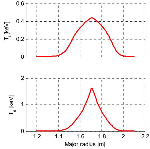
Figure 2. Ion (top) and electron (bottom) temperature profiles of HL-2A.
