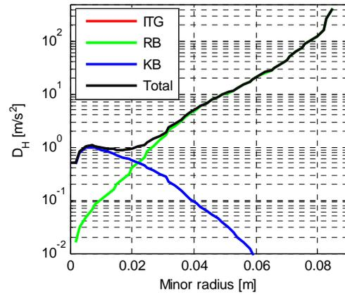
Figure 4. The particle diffusivity plotted as a function of minor radius for ISTTOK.
