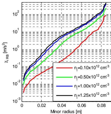
Figure 5. The resistive ballooning contribution plotted for different electron density in ISTTOK.
