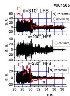
Fig. 2. *The poloidal electric field  $E_{\theta}$ , density  $N_e$  oscillations and the radial fluctuation induced flux  $\Gamma_r(t)$  (red lines) near of the LCFS.*
