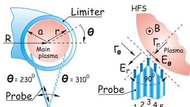
Fig. 1. *Multielectrode Langmuir probe arrangement for measurement at Low (LFS,  $\theta = 310^\circ$ ) and High (HFS,  $\theta = 230^\circ$ ) Field Sides of characteristic properties of periphery plasma parameters.*
