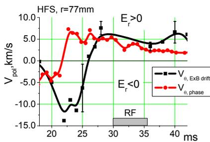
Fig.6 Comparison of the phase poloidal velocity of the periphery plasma fluctuations with  $E_r \times B_\phi$  plasma drift poloidal velocity for long time period of the discharge.
