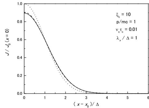
Figure 1: Rf-driven current density in the weak turbulent regime
