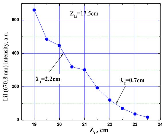
**Fig.3.** The Lithium flux radial distribution in a SOL plasma of T-11M tokamak.
