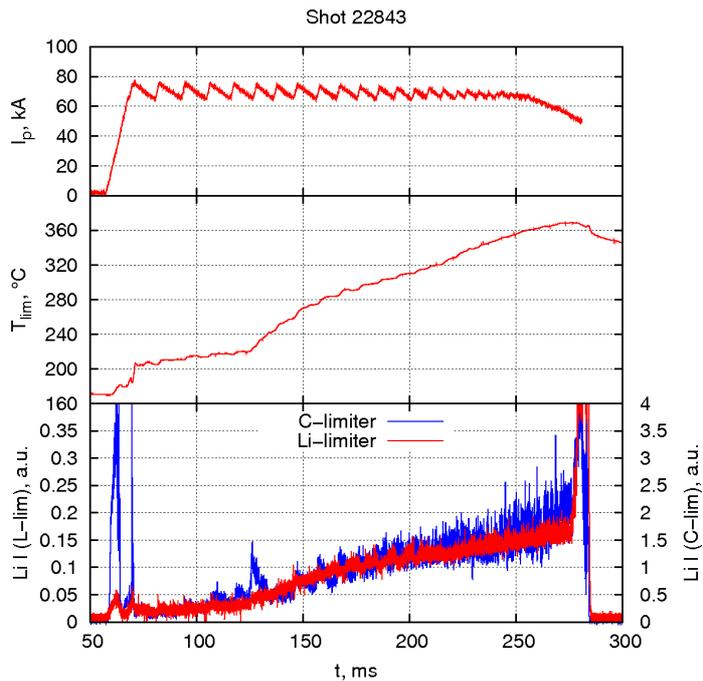
**Fig.2.** The behavior of signals during a tokamak discharge:  $I_p$ -plasma current,  $T_{lim}$  - limiter surface temperature and  $I_{li}$  - intensities from C and Li limiters.
