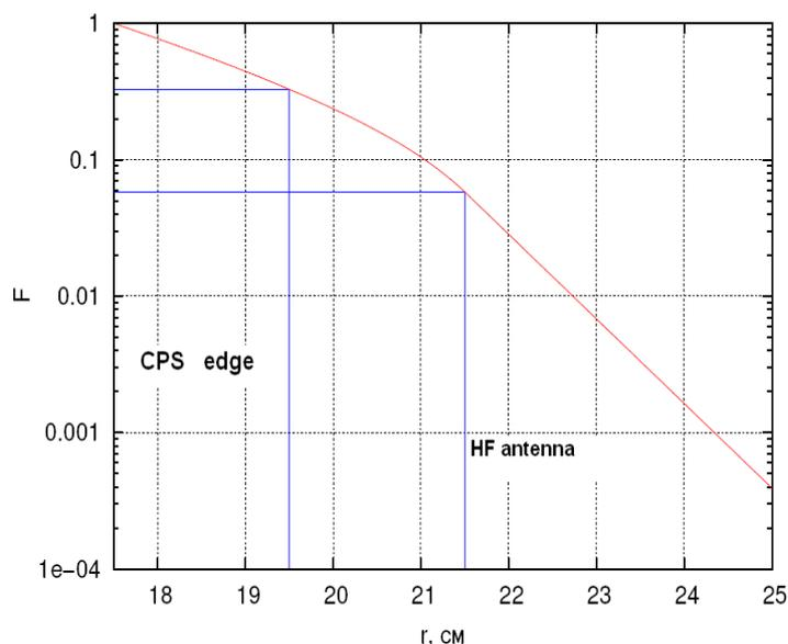
**Fig.5.** The radial distribution function of losses  $F(r)$  for Lithium ions in the T-11M SOL.
