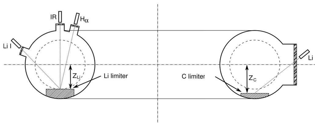
**Fig.1.** The experiment arrangement on T-11M tokamak and optical diagnostics.
