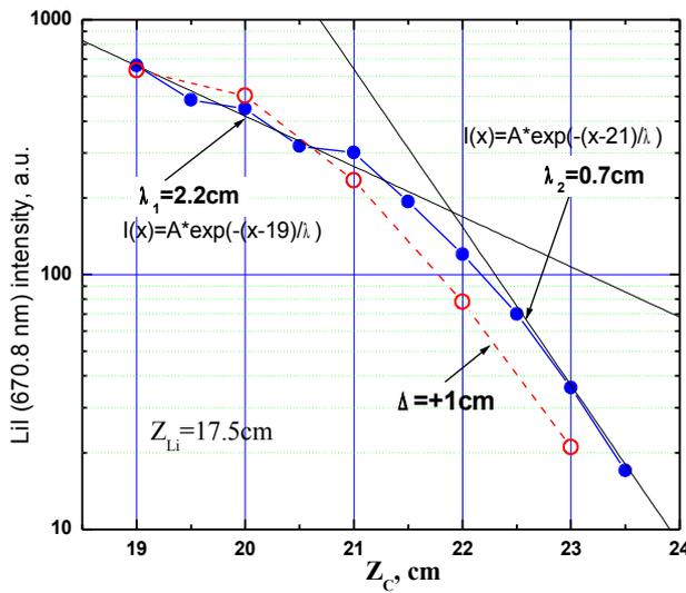
**Fig.4.** The radial distribution of lithium flux cannot be approximated by one exponential fit.
