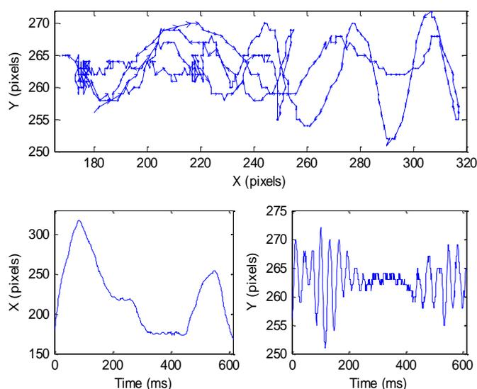
Figure 5: Trajectory of a single particle in a dust cloud showing a different behaviour in x- and y-directions.
