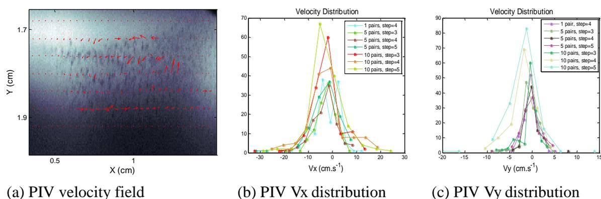
Figure 2: PIV estimation of the dusts velocity field and of the x- and y- components of the velocity distribution, showing the influence of the time interval and number of images pairs considered.
