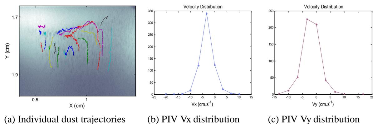
Figure 3: Dusts trajectories and x- and y- components of the dusts velocity distribution, obtained from individual tracking applied to the same data used for PIV calculations in Fig. 2.
