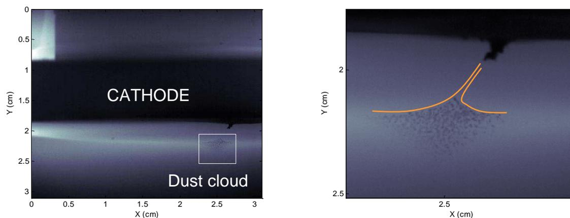
Figure 1: Side view of the cathode showing a dust cloud in the cathode's sheath (left), and detail of the cloud (right). An aggregate made of dusts deposited on the cathode is clearly visible, influencing the shape of the dust cloud.
