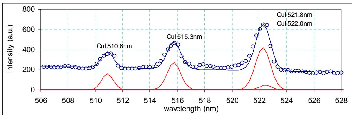
Fig. 3. CuI emission spectrum used for the determination of the electron temperature
