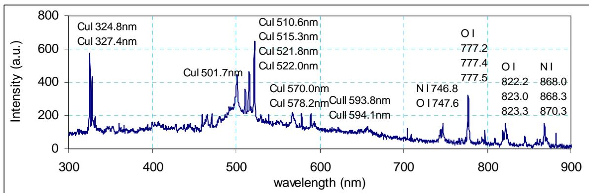
Fig. 2. Emission spectrum of the copper ablation plasma in air
