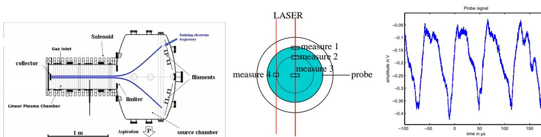
Figure 1: left: sketch of MISTRAL device; middle: measurements points; right: ion density temporal evolution measured by LIF.
