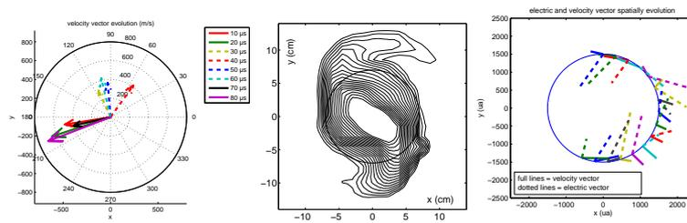
Figure 2: left: ion velocity hodograph; middle: 2D map of the density obtained by probe[2]. The density in the center is higher than the density at the edge. The density is maximum in the arms; right: space reconstruction of ion velocity and electric field. Full lines give the velocity and dotted lines the electric field.
